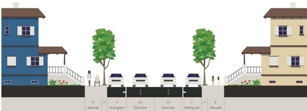
**Figure 3-9: Minor Street - Typical Cross Section, Parking prohibited (44-foot ROW)**
