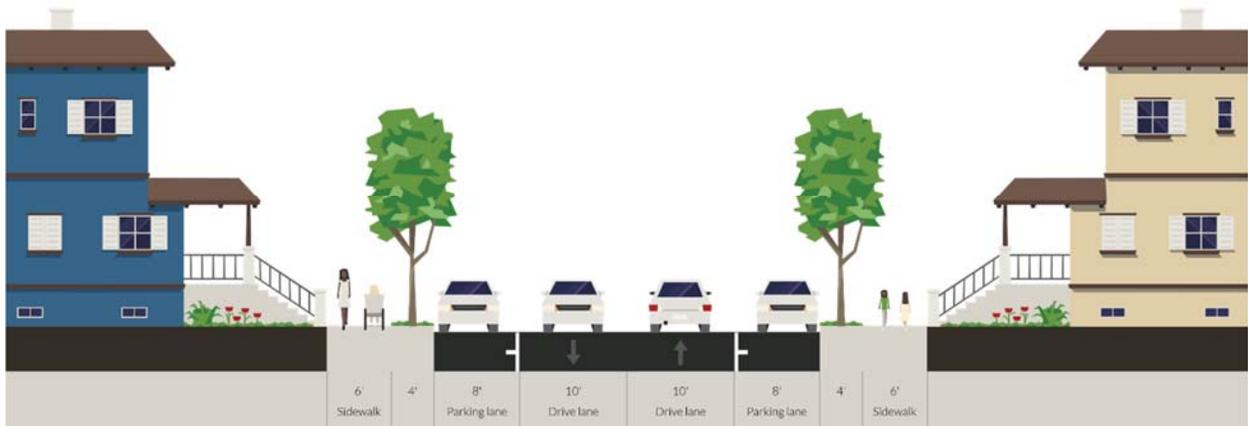
**Figure 3-7: Minor Street - Typical Cross Section, Parking one side (50-foot ROW)**
