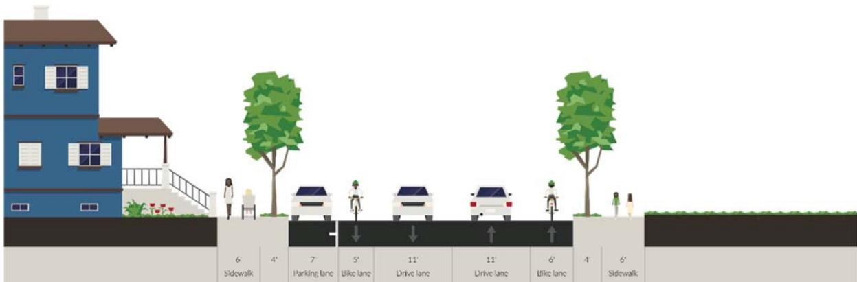
**Figure 3-5: Major Collector - Typical Cross Section, Separated Bike Lanes (70-foot ROW)**
